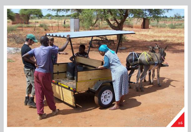
Figure 16: Community members testing the water carrying capabilities of the 'Tin Lizzy' single-axle donkey cart prototype, March 2007.
